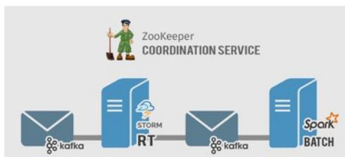
(3) *Coordination service* - While the system is running, ZooKeeper maintains and coordinates the state of data, processes and machines across the various clusters. This helps to ensure the distributed framework behaves correctly and is fail tolerant.
